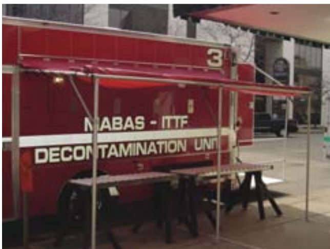
An exterior rehab area allows the vehicles to be used for rehab as well as exterior processing of victims.
