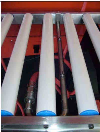
Modec roller system with underside spray boom
